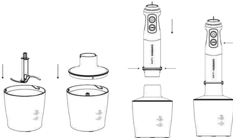
After use unplug then press the ejection button to remove the motor unit. Remove the chopping bowl lid. Carefully take the blade out. Remove the processed food from the chopper bowl.
