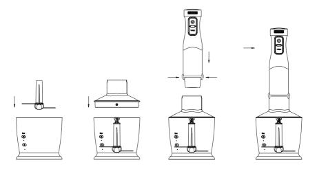
After use unplug then press the ejection button to remove the motor unit. Remove the chopping bowl lid. Carefully take the blade out. Remove the processed food from the chopper bowl.
